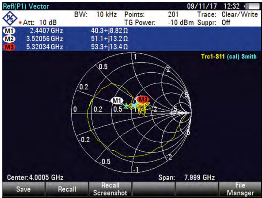
Fig. 9 Measured impedance of proposed antenna
