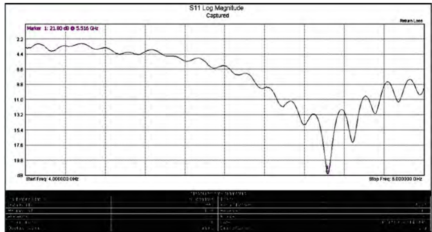
Fig. 14 VNA result of return loss without DGS
