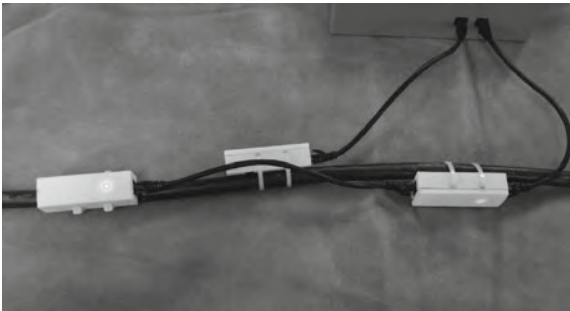
Fig. 4 Experimental model of the contactless power meter. As illustrated in [3, Fig. 16]
